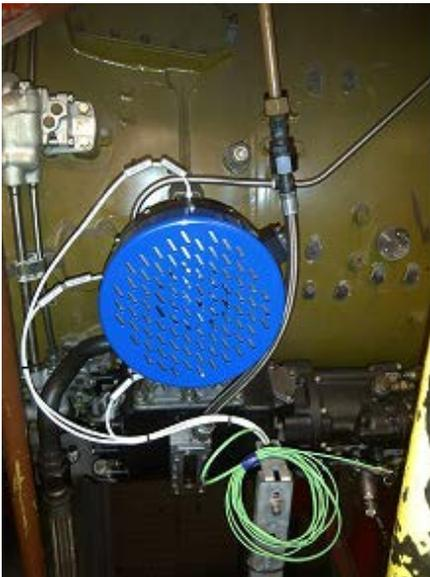
TCL have developed an Anti-windmill brake for use on the RR Avon gas generator. The brake is designed to prevent the Avon turning, wind-milling, whilst shutdown. Wind-milling can occur for a number of reasons:-
