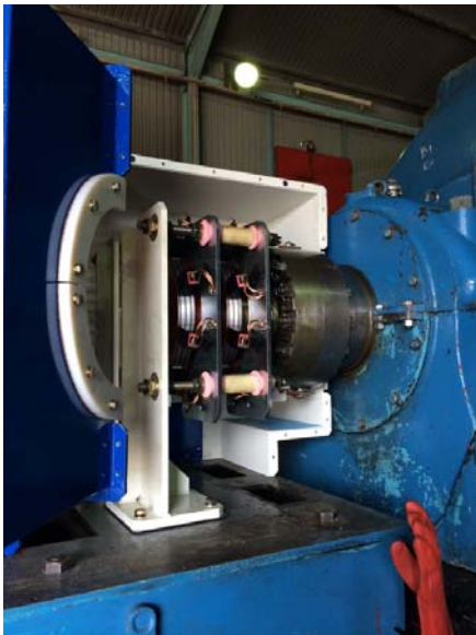
Figure 2 Slip-ring assembly installed
