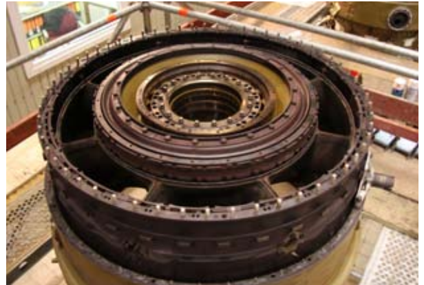
Nozzle box with NGV's removed
